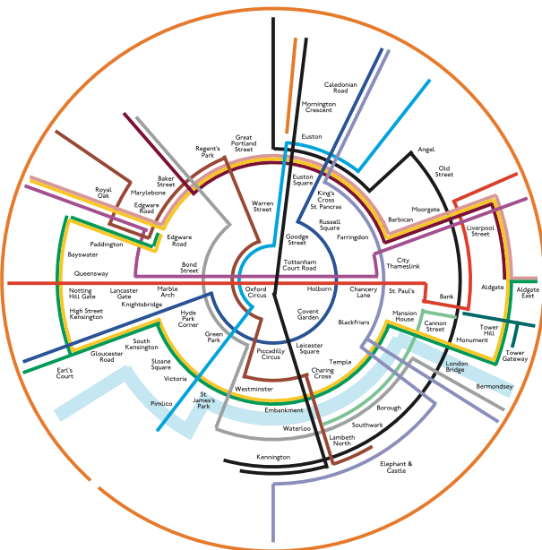
Fig. 6. Prototype London Underground map showing the difficulty with the inner-London Circle Line (yellow). Use of true spokes for its east and west extremities causes these to splay outwards. The path of the Overground loop (orange) is also shown and was prioritised to be a perfect circle for the 2013 concentric circles map (Fig. 7).
